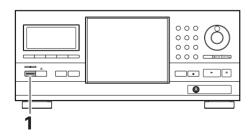
1 Press & (& STANDBY/ON on the front panel).
